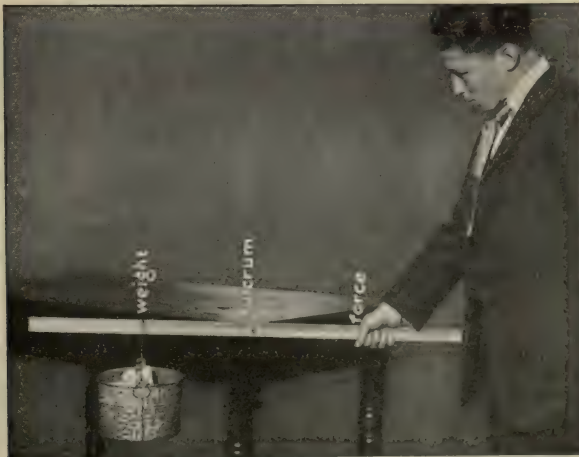
FIG. 27. The yardstick is a lever by which he lifts the pail.
